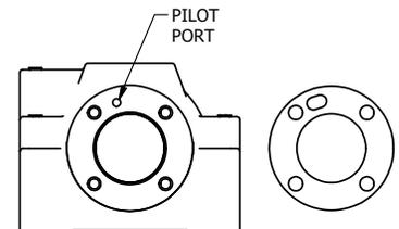
ALIGN PILOT AND HOLE IN GASKET, SIDE 'A' ONLY FOR EXTERNAL PILOT OPERATION - ROTATE THE ROUND ALUMINUM ADAPTOR 180 DEGREES. REMOVE 1/8" NPTF PLUG AND SUPPLY 50-150 PSI TO 1/8" NPTF PILOT PORT IN ADAPTOR.
